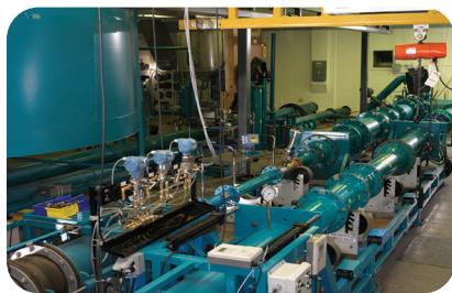
Our Hemet, California factory boasts a robust Calibration Test Lab that enables production of the most accurate and precise flow instrumentation. The test facility utilizes three gravimetric systems and two volumetric systems providing accuracy and calibration tests of flow meters from 15 mm to 500 mm (1/2 to 20-inch) diameter, with flow rates up to 900 m<sup>3</sup>/hr (4,000 gpm).
