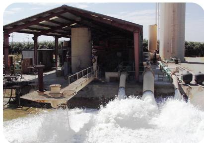
Our large volume test facility is located in Porterville, California. This facility is one of the world's largest volumetric test facilities owned by a meter manufacturer, and it offers accuracy and calibration tests of flow meters from 80 mm to 1,800 mm (3 to 72-inch) diameter, with flow rates up to 13,600 m<sup>3</sup>/hr (60,000 gpm).
